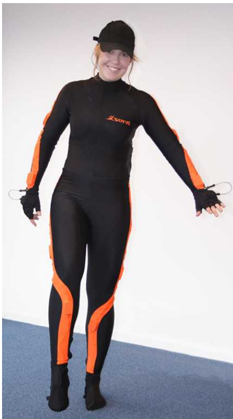
Fig. 1: Human motion capturing suit with inertial sensors (courtesy: Xsens Technologies).
